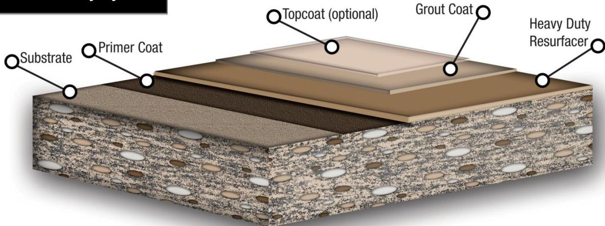
RS-31US is a Water-Based Cement Urethane Slurry Flooring System is a high heat resistant, high strength concrete resurfacing material. The versatility allows use in industries from food and beverage processing to chemical and water treatment facilities requiring a USDA compliant, thermal shock resistant grade floor or when a concrete floor has sustained damage requiring a 3/16” to 1/4” surface restoration.
